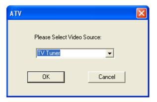
There are four video sources for choice (TV Tuner, FM Radio, Composite and S-Video as in below box) which are up to your Analog devices and drivers.
